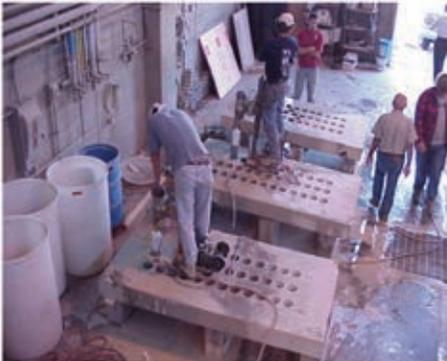
4" x 8" drilled cores.
